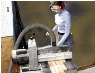
I have to admit that for many years, I did not unplug the table saw when changing blades . Then it dawned on me that it was important to do so, and that if I hung the cord over the hook that holds the wrench, I could unplug and re-plug in the same bending operation. It is the safer way of doing things.
