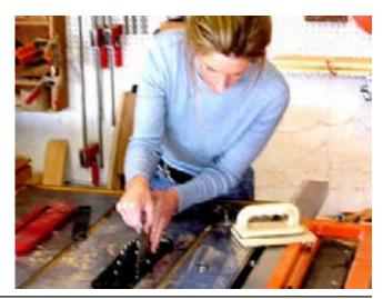
It's time to cut a groove for the front panel and a rabbet for the back.
