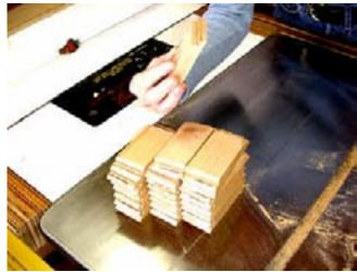
The side pieces were just that much longer so we felt that this hold-down arrangement would work well and be faster than using the jig we used for the vertical pieces.
