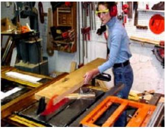
A few minutes later and Beth has the 5 strips we need for the clock cases. Keep in mind, that she moved the fence after each cut, using the blue 5/8" marks on the Incra TS-III template.
