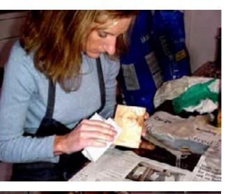
Beth mixes a very small batch of quick curing epoxy. This mix has about 6 minutes working time - just enough for assembling two clock cases.
