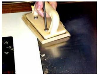
The smaller pieces (4"), that will be top and bottom, are shaped vertically against the fence. Here, Beth loads two pieces in the vertical holding jig I created. The small piece of MDF is used to put pressure on the short pieces from above the jig.
