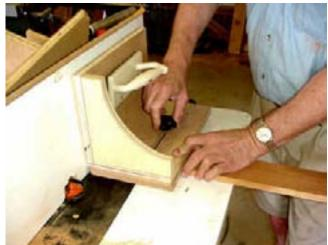
With both pieces cut, I mate them end-to-end. If the router height is exact, the seam between the two will be smooth. If "B" is low, raise the bit.
