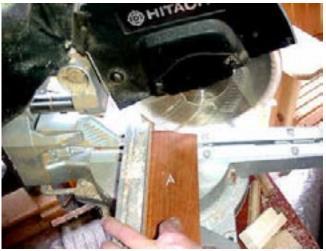
Now for the setting of the fence. At the very beginning, I set the fence so that the stock is even with the front of the bit.
