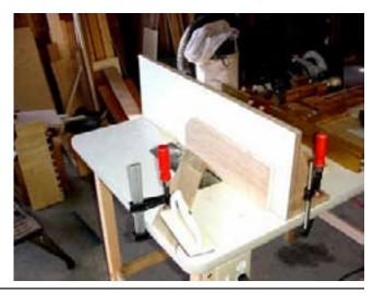
If you try to make perfect adjustments to bit height and fence depth right from the start, it can be confusing. What I do now as standard practice is work on router bit height first, and when that is perfect, I adjust the fence depth.
