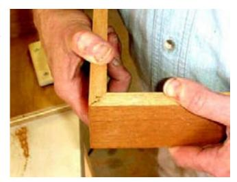
For this set up, I made three test cuts for the router bit height and another three for setting the fence. This photo shows how much stock I used to make these cuts (5" total). Not a bad price to pay for a perfect joint.
