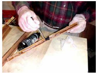
On the mating piece, I moisten the surfaces with a brush dipped in water. The water activates the polyurethane glue and makes for a tighter bond.
