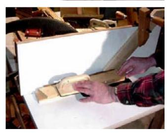
The 4 pieces fit together very well. By dry fitting them, you can see if there is any adjustment that needs to be made before glue up.
