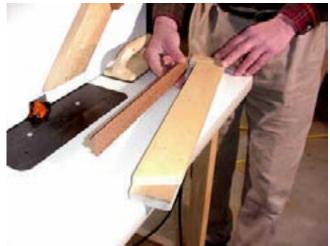
The second part of the solution is to cut the stock 2" longer than will be needed. I found that if I were very careful at the end of each pass, I could minimize the amount of movement, and therefore reduce snipe...but there is no guarantee, so allowing the extra inches makes sense to me.
