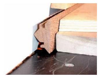
My answer to the problem is two part: 1) I made a simple push-stick that would fit the entire length of the stock and would bear pressure on the vertical mid-point. The end of the push-stick has a cut-out to grab the end of the stock...giving me better feed control.
