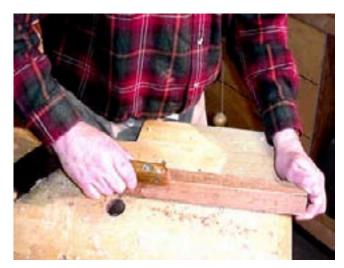
The finished leg is perfect in fit and is very strong—in fact, it should be stronger than a leg cut from one piece (at left). It certainly looks good with all four sides having edge grain. I did add a bit of wood putty to where the fit wasn't exact near the end of the piece.
