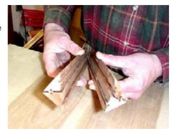
I used polyurethane glue for this leg. There is a great deal of gluing surface. I carefully brushed the glue into every surface on one piece.
