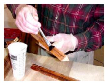
When the two pairs of sections are glued, I then apply glue to them and position them together.
