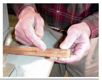
The second edge of each piece will be routed flat against the fence. While at the beginning, there is enough flat surface for the piece to be steady, at the end of the cut, the stock is only resting on the cut apex and can easily swivel away from vertical.
