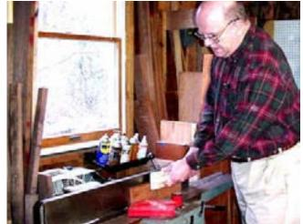
I then cut them to exactly  $1\ 1/2$ " width. You might be tempted to make this width a bit proud and then run the 2nd side through the jointer, but that isn't necessary. The ripped edge will be removed in the running of the locking miter bit shape, and my ripping blade gives me a very smooth cut.
