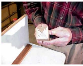
I also found that if you assemble them in order, the last joint is difficult to bring together. A better way is to assemble two sets of two sections...and then put those together to make the completed leg.
