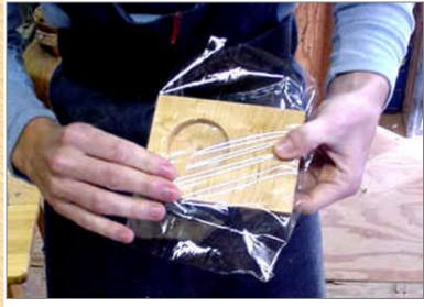
With the clock panels totally dry, Beth wraps them in Saran Wrap. This will keep the cherry stain and finish from ruining these face panels. The thickness of the plastic wrap will not interfere with the panels being placed in the case dados.
