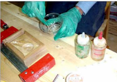
Beth mixes a very small batch of quick curing epoxy. This mix has about 6 minutes working time just enough for assembling two clock cases.
