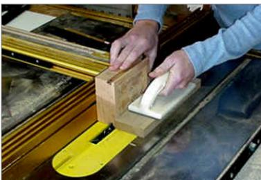
Deciding that the two sides should be at an angle of 15°, Beth has installed the stacked dado set and set the blade tilt angle to 15°. She uses a push shoe to guide the box over the dado set.
